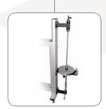
**HVT12b** - Torsional Oscillation (Free and Damped) Module
