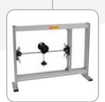
**HVT12c** - Beam Bending (Transverse) Vibrations Module
