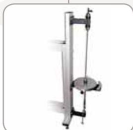
HVT12b - Torsional Oscillation (Free and Damped) Module
